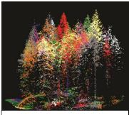
Segmented Tree LiDAR Point Cloud
